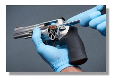
Attach the brush attachment to the cleaning rod, apply bore cleaner to the brush and insert assembly in the barrel from the front to clean the bore. Using the same attachment assembly, insert in the chamber from the back. Make sure use the in and out method to clean the residue from the barrel and the chamber.
