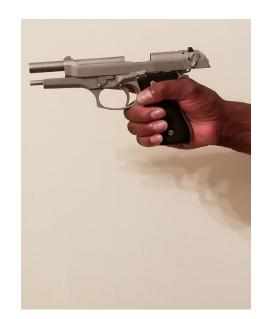
With the slide fully rearward engage the slide lock to visually inspect the chamber to ensure that it is empty. If the firearm is to be put back into its case release or ease the slide forward. Depending on the type of pistol make sure the hammer is not cock by utilizing the decocker or by pulling the trigger on the empty chamber.
