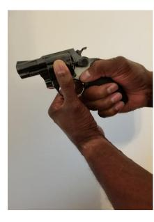
Once the cylinder is full, position the revolver back in the right hand and then push the cylinder back into the frame with the left hand thumb. The revolver is ready to fire.
