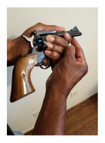
Release the ejector rod when the case or cartridge is exposed. Remove the case or cartridge and rotate the cylinder to the next chamber. The process is repeated until the chambers are empty.
