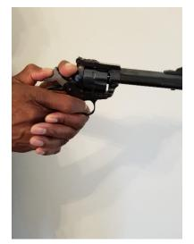
Position the support hand thumb between the hammer and the firing pin plate of the gun. Position the shooting hand finger on the trigger and press. The support hand thumb is there to prevent the hammer from striking the firing pin and firing the gun when the trigger is pressed.
