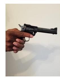
Ease the hammer all the way down and then remove thumb from the hammer spur. Maintain the gun pointing in a safe direction.
