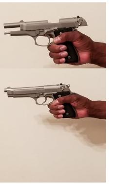
Always point your gun in a safe direction. Loading can be accomplished with the slide open or closed. In the close position the shooter will have to retract the slide to the rear and release; like a sling shot, the slide will remove a cartridge from the magazine and insert it in the chamber.
