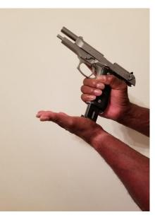
Insert the magazine, normally a click is heard when the magazine is fully seated. To ensure the magazine is seated properly tap the floor plate/base of the magazine into the pistol.
