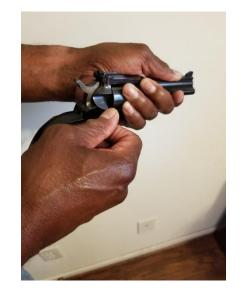
Open the loading gate with the right thumb. In some models the hammer is placed in the half-cocked position at this stage for the cylinder to rotate during loading. This model doesn't need to be in the half-cocked position for the loading process.
