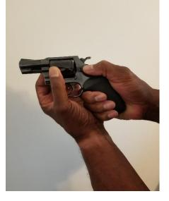
Always keeping the gun pointed in a safe direction. With the revolver held in the right hand (for both right and left handed shooters) and finger off the trigger use the right hand thumb to engage the cylinder latch release.
