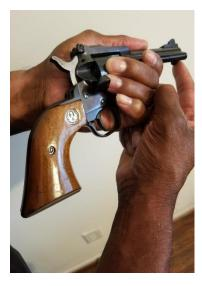
Align the empty case or live cartridge with the loading gate. The index finger of the shooting hand engages the ejector rod and pulls the rod rearward to push the case or cartridge out of the chamber.
