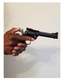
Remove the shooting hand finger off of the trigger while controlling the lowering of the hammer with the thumb all the way to the gun.
