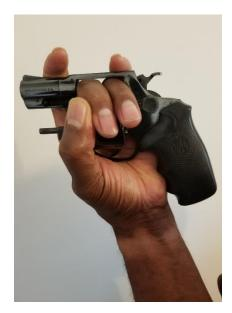
While the cylinder latch release engaged push out the cylinder from the frame with the left hand fingertips. Maintain a good hold on the revolver to start the loading process.
