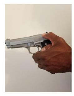
With the support hand thumb engage the safety/decocker to lower the hammer which prevents the firing pin from being struck by the hammer when it contacts the frame area.
