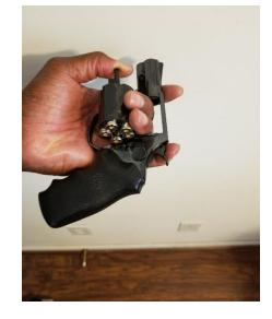
While the cylinder latch release engaged push out the cylinder from the frame with the left hand fingertips. Maintain a good hold on the revolver to start the unloading process. Position the left hand thumb on the ejector rod.
